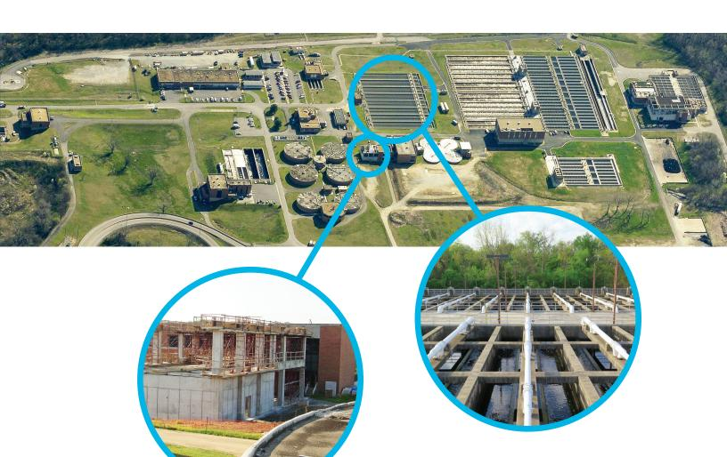
Contract 3 consisted of the construction of scum collection troughs and motor-operated scum gates in the preliminary sedimentation tanks for scum removal, installation of scum chopper pumps, and the construction of a new two-story building to house new scum concentration equipment and bio-trickling filter and activated carbon odor control equipment.
