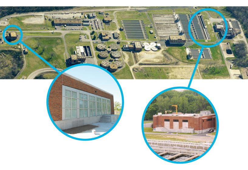
Contract 2 consisted of the construction of a new ultraviolet (UV) disinfection facility to replace the existing chlorine gas disinfection and sulfur dioxide dechlorination system and the upgrading of the main plant switchgear and electrical distribution system to improve reliability of power feeds to all plant facilities.
